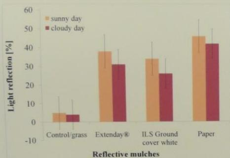
Fig. 1: Relative light reflection of different reflective mulches on a sunny and a cloudy day [%].
